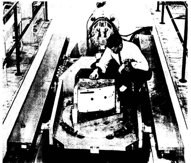
**SHOCK TEST** — Gemini prototype computer is prepared for rugged impact shock test on IBM's High-G sled in Owego, N.Y. Sled can test units from 15-g's up to 100-g's.
